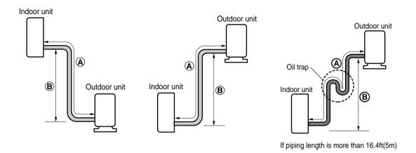
CAUTION: Capacity is based on standard length and maximum allowance length is on the basis of reliability.
